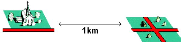
$$\begin{aligned} \frac{\text{Distance on the Map}}{\text{Distance on the Ground}} &= \frac{2 \text{ cm}}{1 \text{ km}} = \frac{2 \text{ cm}}{100\,000 \text{ cm}} \\ &= \frac{1}{50\,000} \\ &= \mathbf{1/50\,000 \text{ Scale}} \end{aligned}$$
