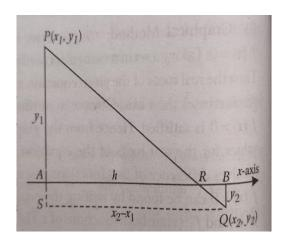
we find  $y^{(1)}$  by  $y^{(1)} = f(x^{(1)})$ . Now either  $y^{(1)}$  and  $y_1$  and  $y_1$  and  $y_2$  will be of opposite signs. If  $y^{(1)}$  and  $y_1$  are of opposite signs then one root lies in the interval  $(x_1, x^{(1)})$ . We again apply the method of false position to this interval and get the second approximation.
