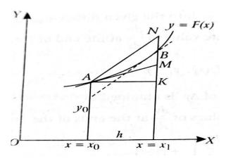
In this figure KM represents the  $\Delta y$  computed by the Euler method. if AN is drawn parallel to the tangent at B, then KN represents
