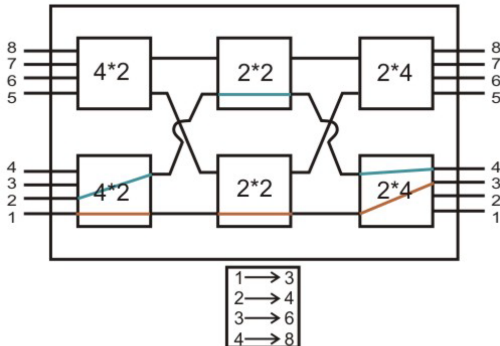
Figure 2.6 Block nature of the switch
