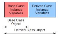
A derived class object contains the instance variables of the base class and those of the derived class, while a base class object only contains the instance variables of the base class.
