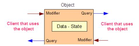
Every member function has direct access to the data members of its class as well as its other member functions. Each member function receives and passes information between the client and its object through parameters and a return value.
