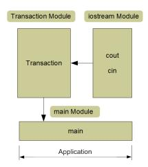
To translating the source code of any module the compiler needs information identifying the names used in that modules but defined outside the module. To enable this, we store C++ source code for each module in two separate files:
