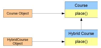
Operations that are identical for all of the types within the hierarchy require only single definitions. The *assessments()* query on a *HybridCourse* object invokes the same logic as one on the *Course* object. Defining a query for the *HybridCourse* class would only duplicate existing code. Inclusion polymorphism eliminates duplicate logic across a hierarchy.
