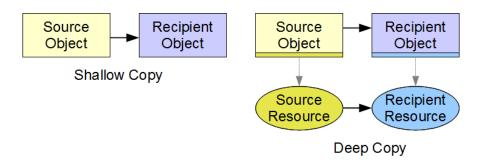
For each deep copy, we allocate memory for a new resource and copy the contents of the original resource into that new memory. We shallow copy only those instance variables that are NOT
