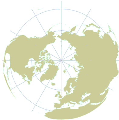
Fig. 3.23: Polar azimuthal orthographic projection.
