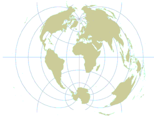
Fig. 3.20: Polyconic projection, with true scale along each parallel.
