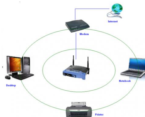
Figure 44: A typical Wireless network
