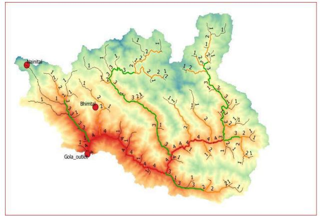
Fig.6.16 Stream order of Gola watershed with outlet at Kathgodam, Nainital
