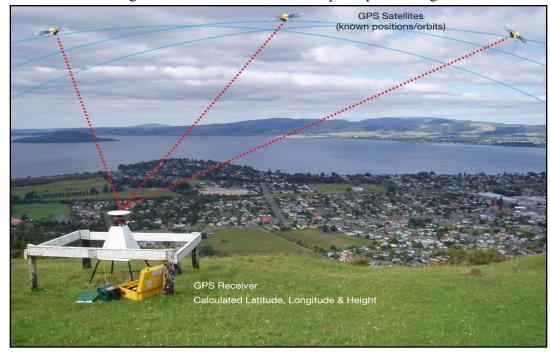
Figure 10.3 GPS receiver and its point positioning
