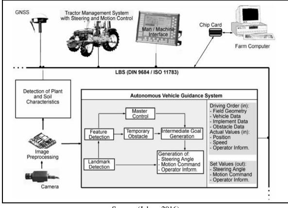
Figure 8.7 Standard Guidance system hardware construction
