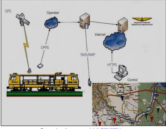
Figure 12.5 System for safety and protection of Railways
