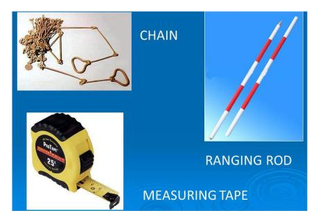
Figure 8.6 Instruments used for Direct Measurement
