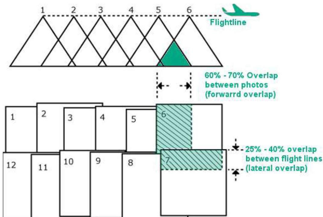
Fig 4.6(b) Overlap required to get the full coverage of area
