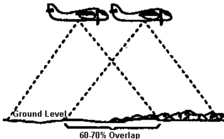
Fig 4.6(a) Overlap required to get the full coverage of area
