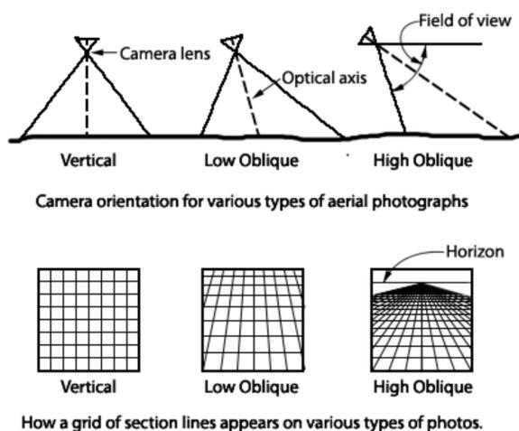
Fig 4.8(a) Camera orientation for various types of photograph
