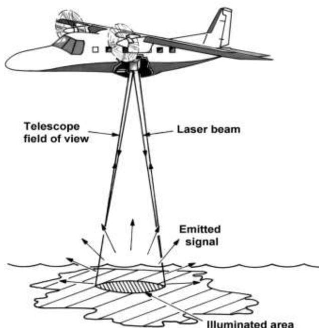
Fig 4.5. Flight direction and signal receiving process
