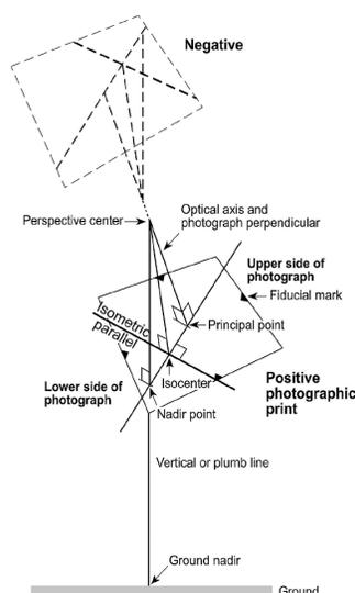
Fig.7.9 Plumb point or nadir point , Isocentre and principal point
