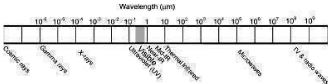
**Figure 2.9 Electromagnetic Spectrum of all Specific wavelength Regions**
