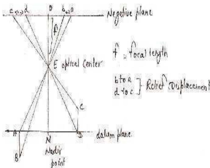
Fig. 6.15 Height of object in relation to datum plane
