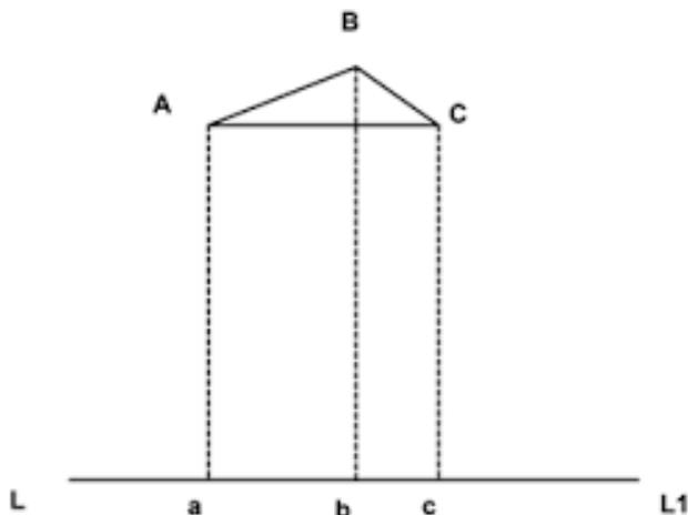
Fig.7.2 Orthogonal Projection
