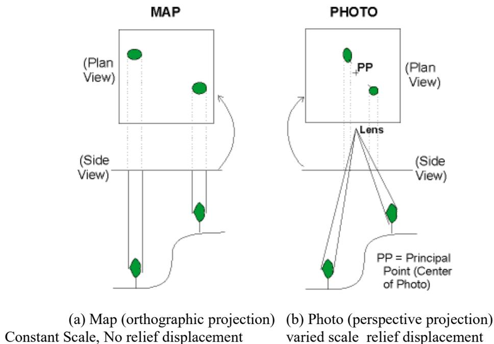
Fig. 6.6 Comparative geometry of (a) map and (b) a vertical photograph, differences in shape, size and location of the two trees.
