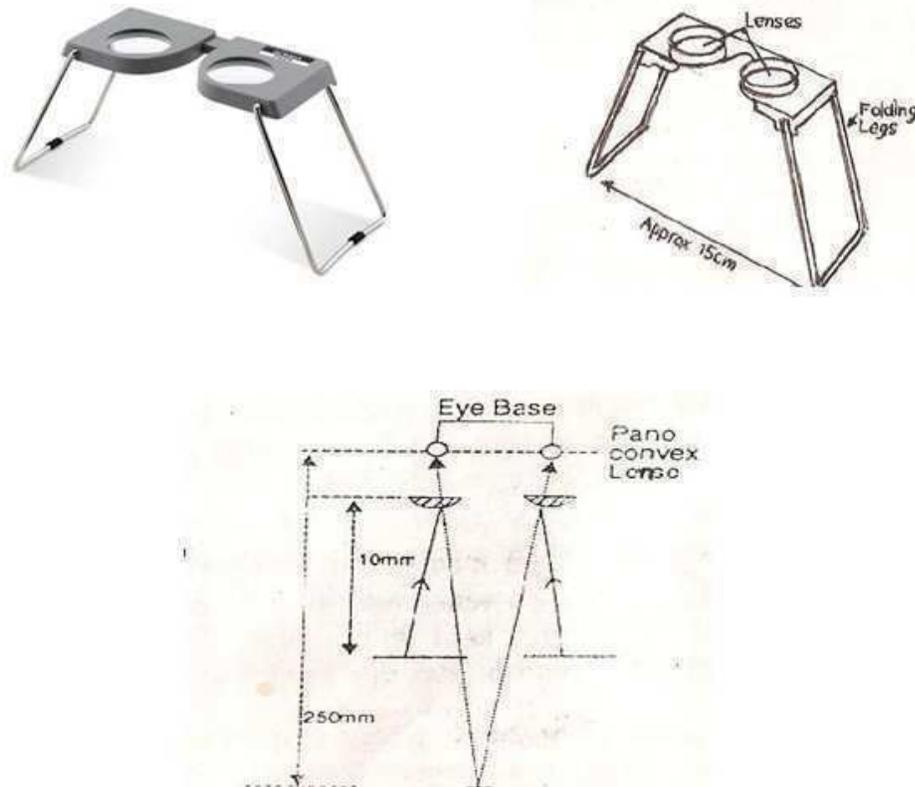
Fig.5.3 pocket or Lens stereoscope (Source: Girard, 2003)
