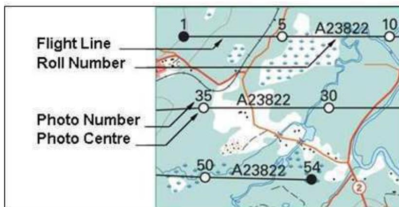
Fig.7.5 Flight line and index map
