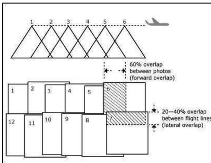
Fig.7.10 Forward and lateral overlapping
