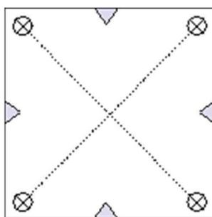
Fig.7.6 Location of the fiducial marks and principal point for an aerial photo image. The intersection of the dotted line indicates the principle point.
