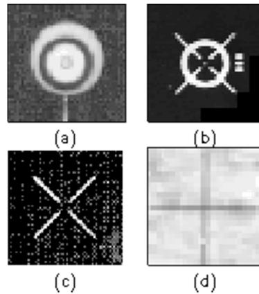
Fig.-7.7 Several typical shapes of fiducial mark in an aerial photo image.
