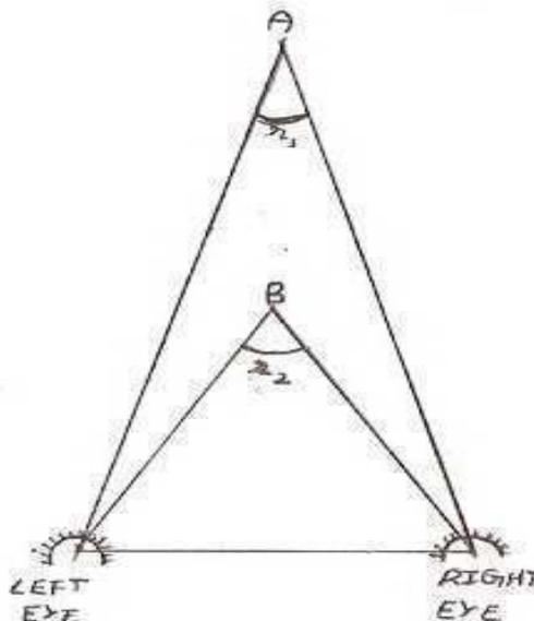
Fig 5.2 Converging Angle in viewing object at different distance (Devi sunita, 2012)
