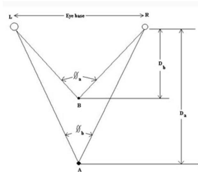
Fig.5.1 Human stereoscopic vision
