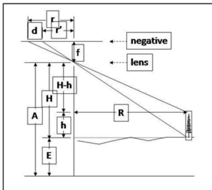
Fig.7.13 Relief Displacement
