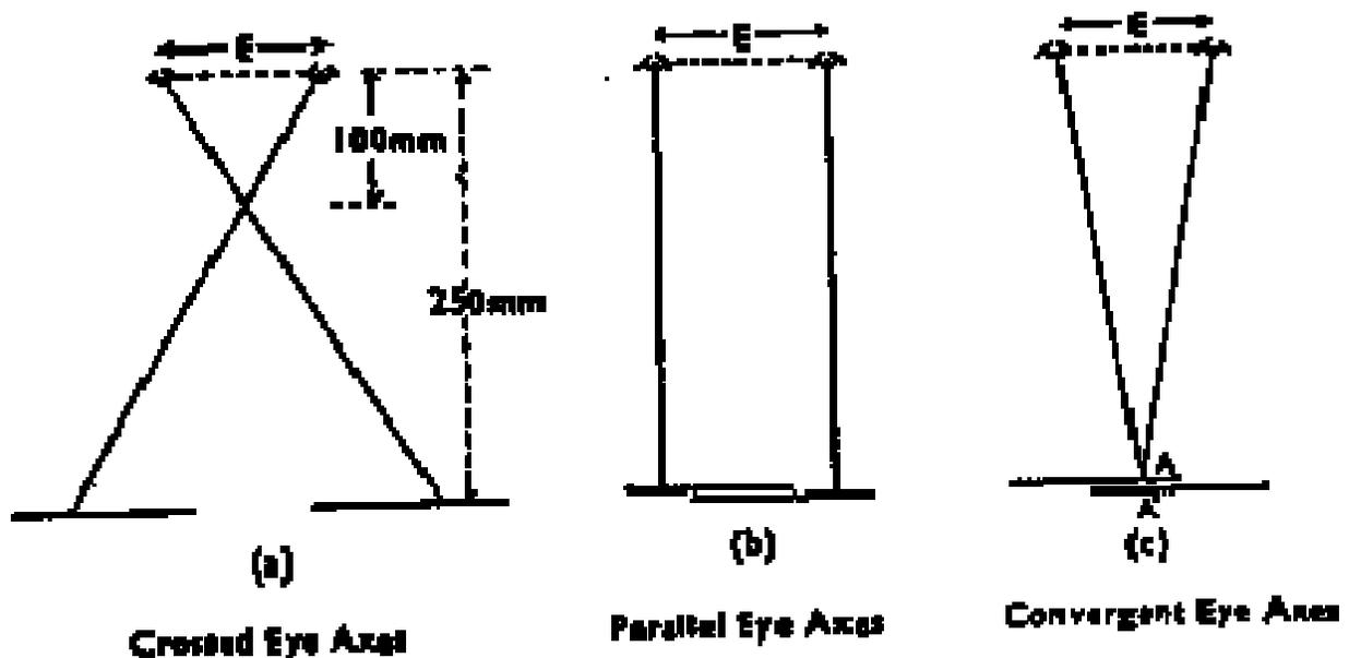
Fig.5.7 Three ways of looking at stereoscopic photographs
