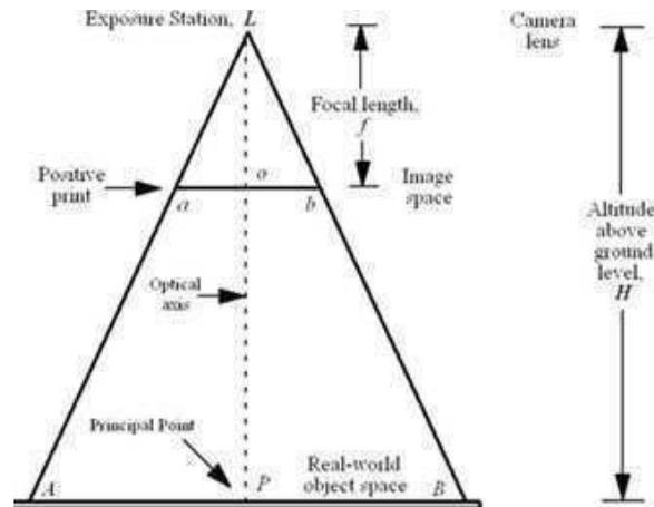
Fig.7.12 Relationship Between the Focal Length ( $f$ ) and the Aircraft's Flying Height ( $H$ ):
