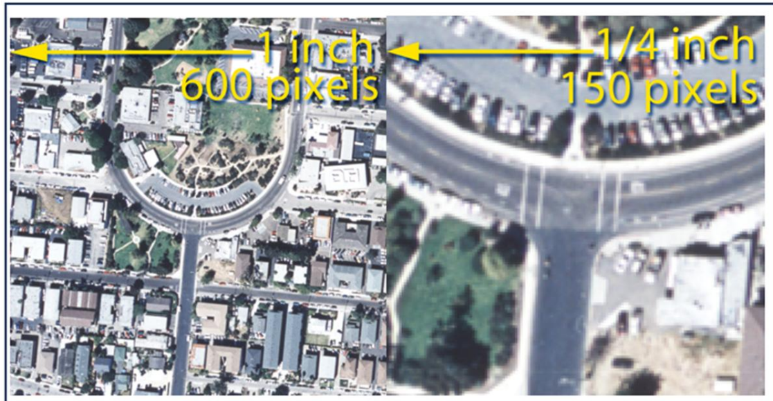
Fig. 4.2: Aerial Photograph Ground Coverage, Resolution and Scale.
