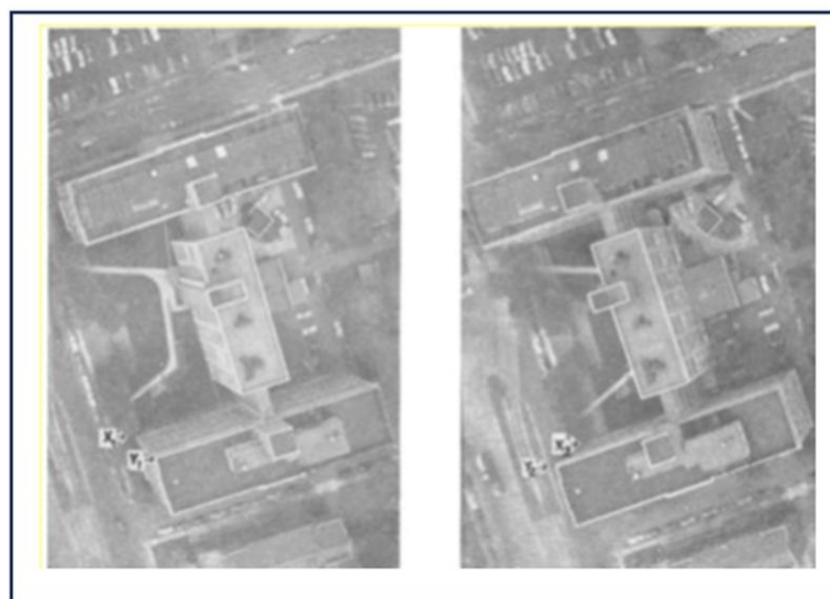
Fig. 2.16: Aerial Photos Showing Image Parallax.
