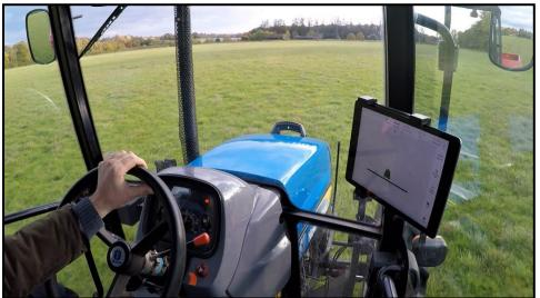
Figure 5.6 Tractor Guidance through GPS
