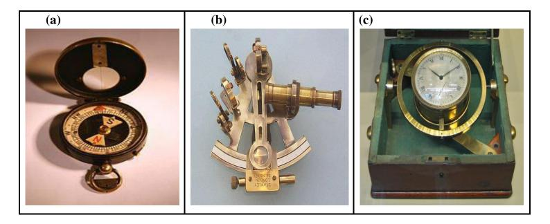
Figure 9.2 Ancient Navigation tools a) Magnetic Compass, b) Sextant, c) Chronometer
