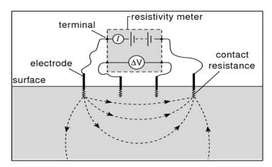
Fig.3.8 Components of Resistivity Meter
