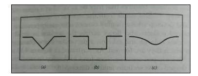
Fig 2.7 Illustrative gully cross sections: (a) sand and gavel;(b) silt; (c) silty clay or clay
