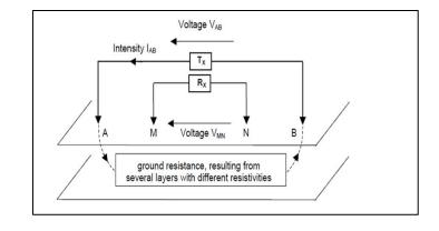
Fig. 3.9 Ground resistance, resulting from several layers with different resistivities
