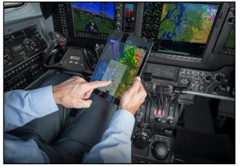
Figure 9.4 GPS showing the navigation route in cockpit monitor
