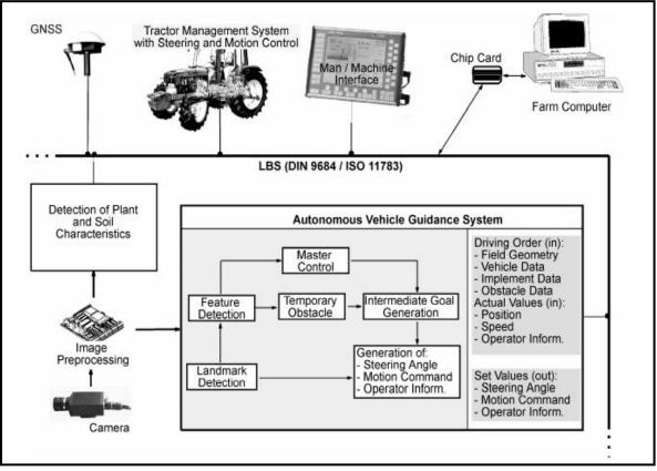
Figure 5.7 Standard Guidance system hardware construction
