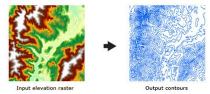
Fig. 2.2 A contour map is generated by using DEM
