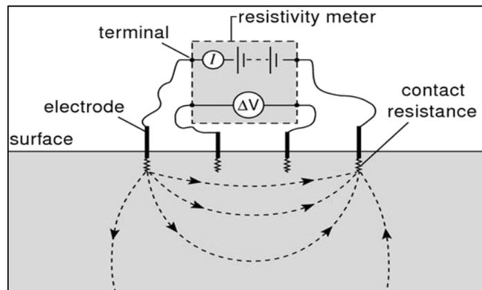
Electrode Layouts of Schlumberger Array – Generally used for VES.
