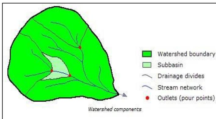
Fig. 6.15 components of drainage system
