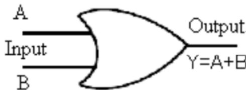
**Figure 3: Graphical symbol for OR gate**
