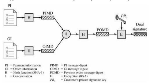
Figure 5.2: Construction of Dual Signature
