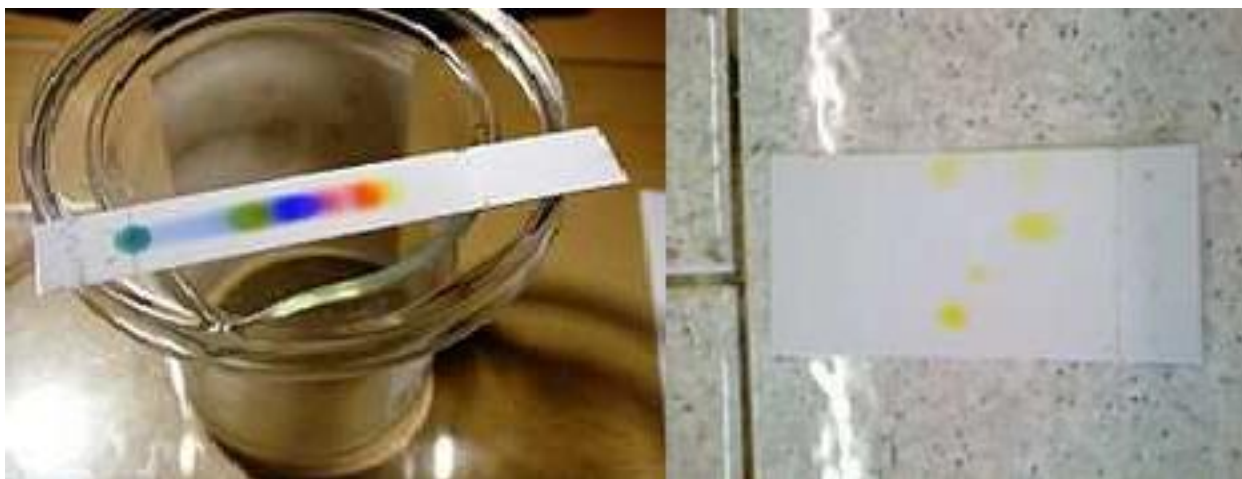
Fig.7.22 Separation of black ink on a TLC plate
