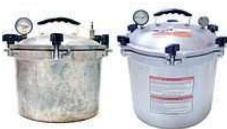
Fig 7.5 Stovetop autoclaves—the simplest of autoclaves
