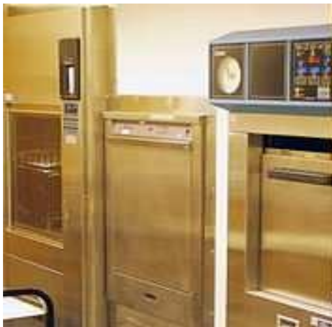
Fig 7.6 The machine on the right is an autoclave used for processing substantial quantities of laboratory equipment prior to reuse, and infectious material prior to disposal. (The machines on the left and in the middle are washing machines.)
