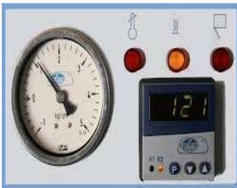
Fig 7.7 The Autoclave must reach 121 degrees Celsius
