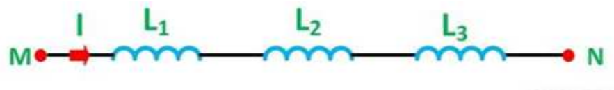
Figure 2.12: Inductor in series.
