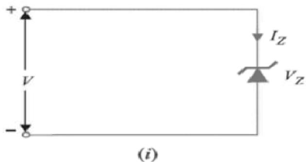
Figure 3.30: Equivalent circuit of Zener for "ON" state.
