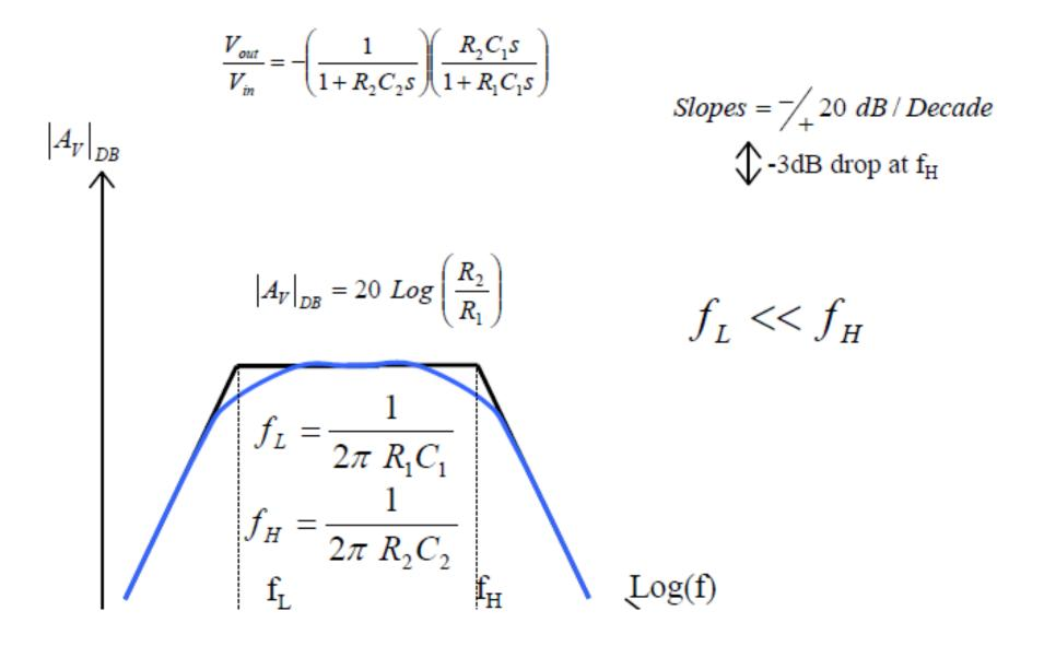
Band Pass Filter (combination of high and low pass filter)
