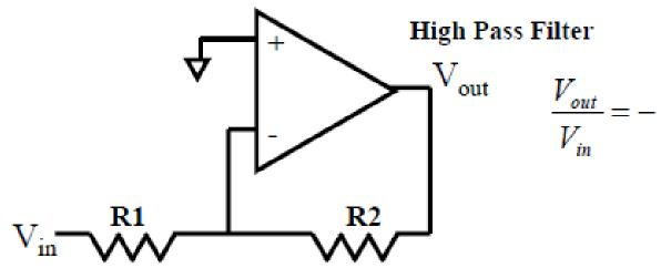
$$\frac{V_{out}}{V_{in}} = -\frac{R_2}{R_1}$$
