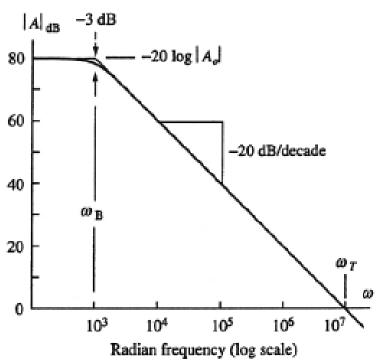
$$\left|A_{OpenLoop}(j\,\varpi)\right| = \frac{A_{O}\,\varpi_{B}}{\sqrt{\varpi^{2} + \varpi_{B}^{2}}}$$
