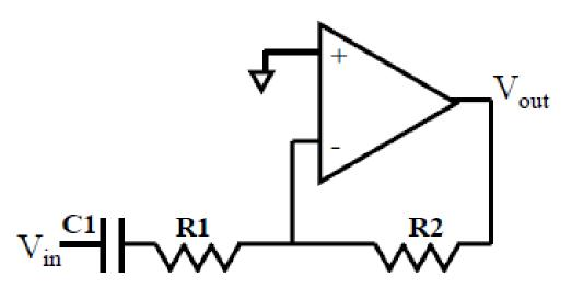
$$\frac{V_{out}}{V_{in}} = -\frac{R_2}{R_1 + \frac{1}{C_1 s}}$$
