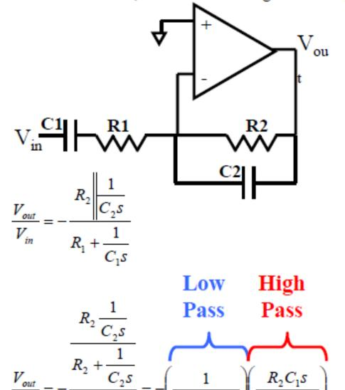
Band Pass Filter (combination of high and low pass filter)
