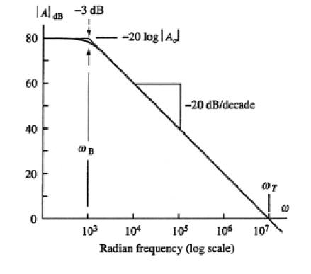
$\varpi_T \equiv \text{Unity - gain frequency (frequency where } |A_{OpenLoop}(s)| = 1)$
