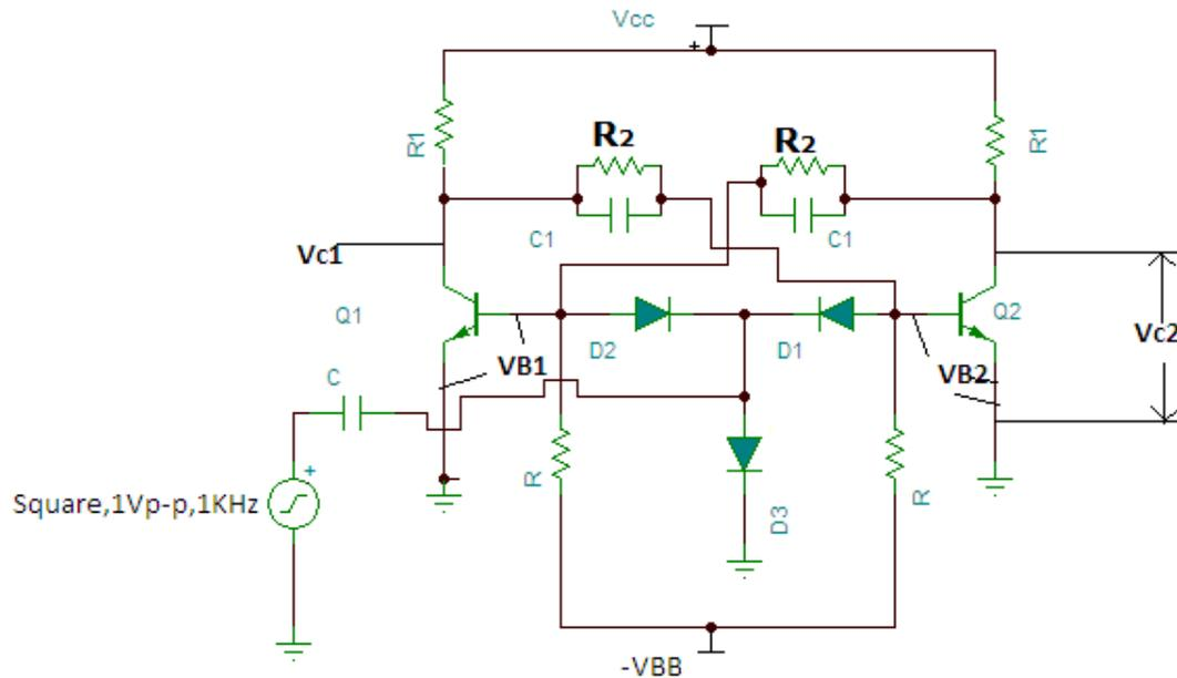
When VCC is applied, one transistor will start conducting slightly more than that of the other. Let Q2 be ON and Q1 be OFF.
