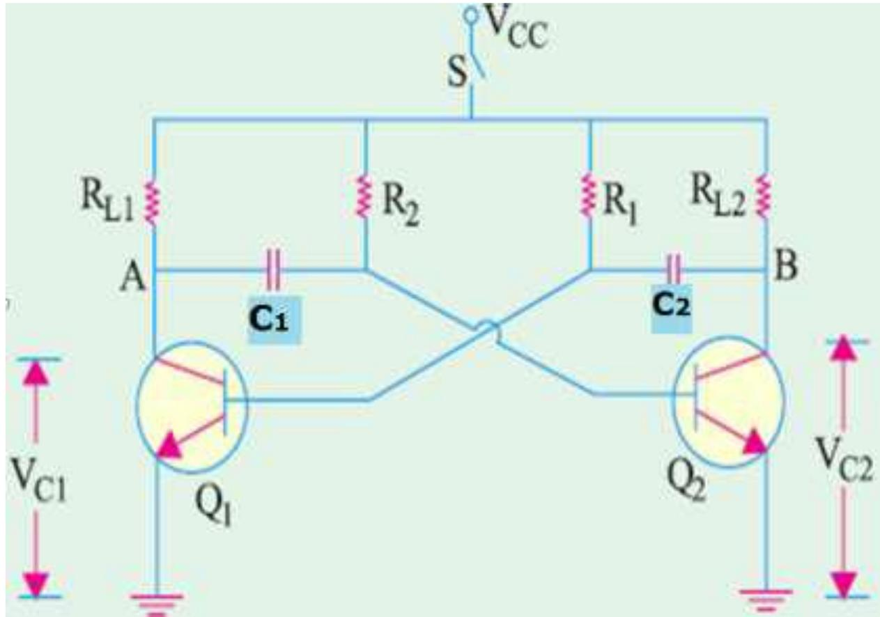
This astable circuit consists of two transistors, a cross coupled Feedback network, and two capacitors and four resistors.
