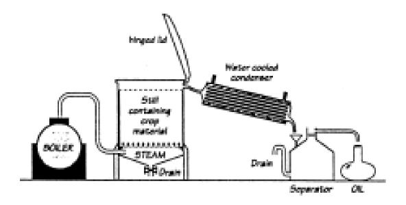
Fig. Basic still design for steam distillation
