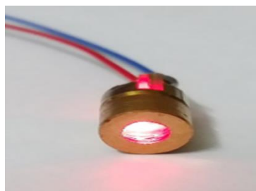
Figure: 6.2: A simple and low power metal enclosed laser diode
