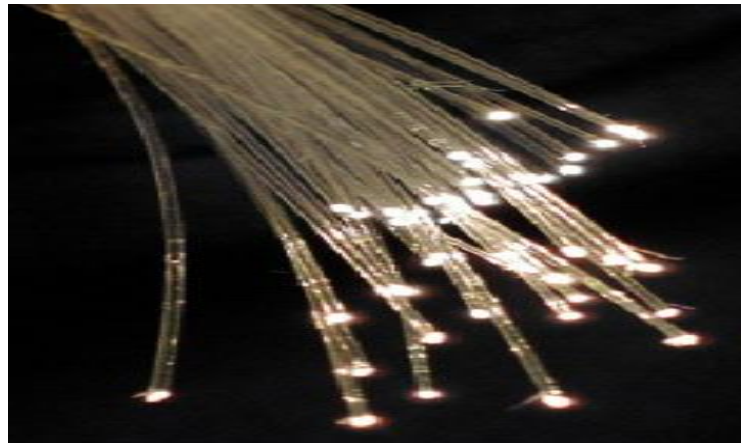
Figure: 7.1: A Bundle of optical Fiber
