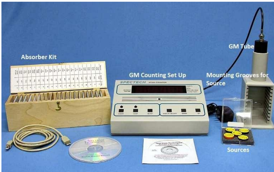
Figure 3: Experimental set up for GM Counter based experiments. Taken from the company manual http://www.spectrumtechniques.com/resources/instrument-manuals/
