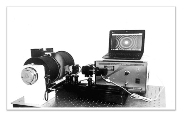
Figure 1: A setup of the Zeeman Effect on a vibration less table
