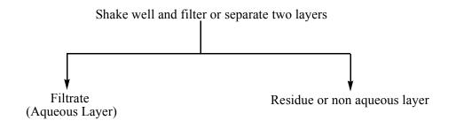
Cool the aqueous layer (filtrate) in an ice bath and add cold 10% NaOH solution drop-wise till the solution becomes alkaline. Cool the resulting alkaline solution in an ice bath.
