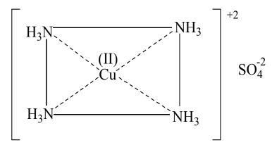
Structure of tetraammine copper (II) sulphate ([Cu(NH<sub>3</sub>)<sub>4</sub>]SO<sub>4</sub>)
