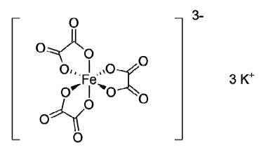
Structure of potassium trioxalato ferrate (III) complex
