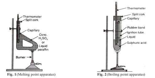
The flask is gently heated from the point shown and rise in temperature is observed carefully. The temperature at which the substance begins to liquefy is noted. The temperature at which the solid has completely changed into liquid is also noted. This range of temperature is recorded as M.P. range of the substance. In case compound is pure, the melting point is quite sharp and occurs over 0.5 to 1°C range of variation. During melting of the solid, the temperature remains constant.
