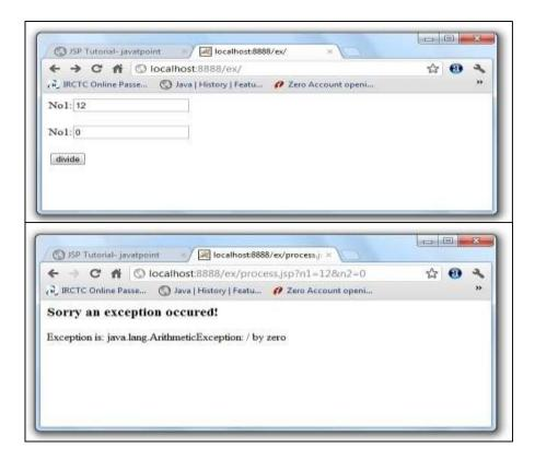
Figure 4. Output for division when an exception occurred (using Exception Handling)
